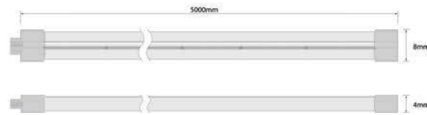
-RUBBER LED STRIP 6W/m IP67
